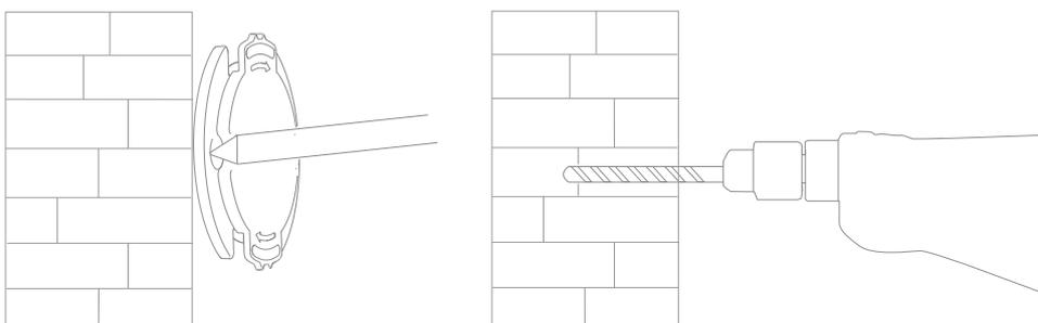
2. Insert the two plastic anchors into the holes on the wall.
